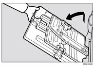
**2** Lift the paper delivery side plates and adjust them to the paper size.
